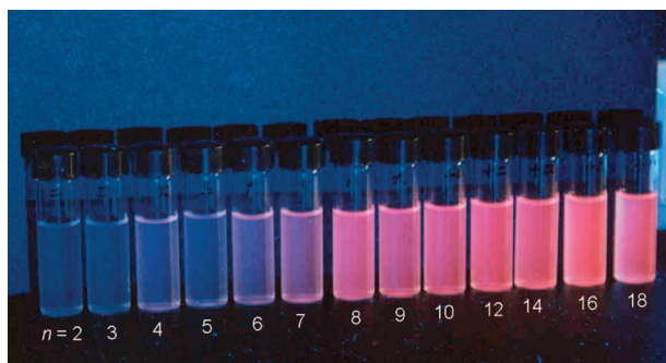
Figure 4. Photograph of the luminescence of the Au(I)–SRs (excited by longwave UV \geq 350 nm, Black Ray longwave ultraviolet lamp model B100 AP, UVP Inc.) dispersed in THF.
